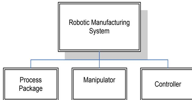
Figure 13. Start-up Visionary WBS for a Robotic Manufacturing System
