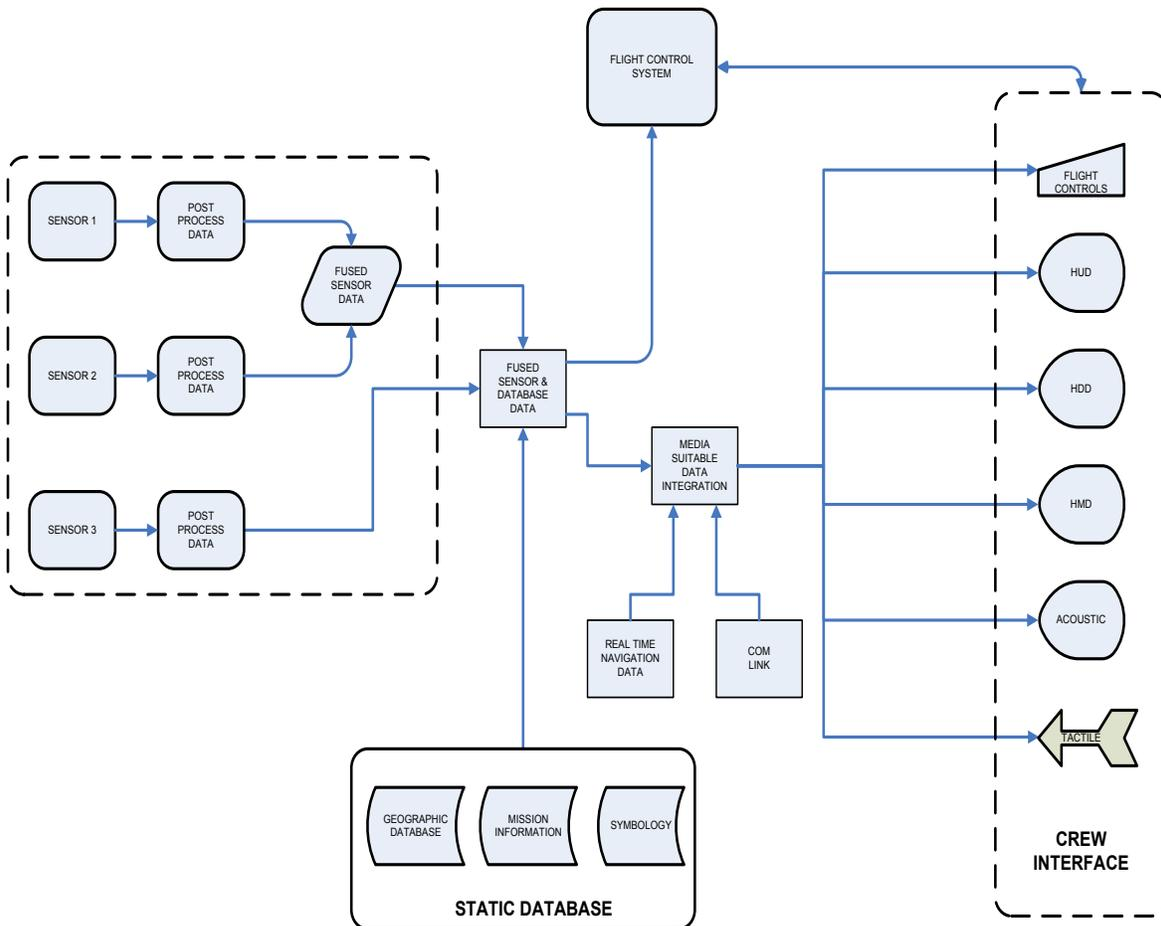
Figure 12. Notional Architecture for a Flight Control System; an Example of a Simple Architecture not in WBS Format
