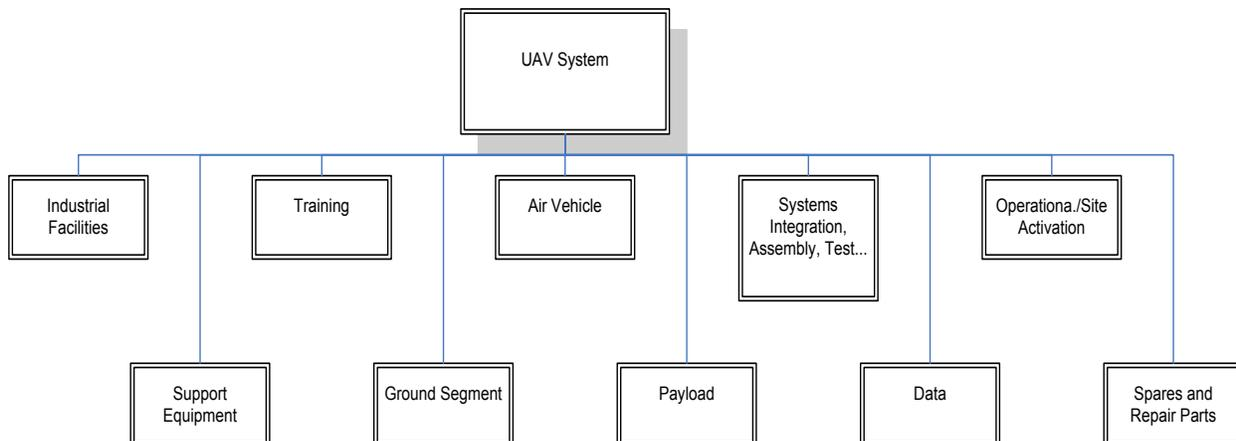
Figure 10. UAV System Top-Level WBS Based on MIL-HDBK-881A, Appendix H, H.3 Work Breakdown Structure
