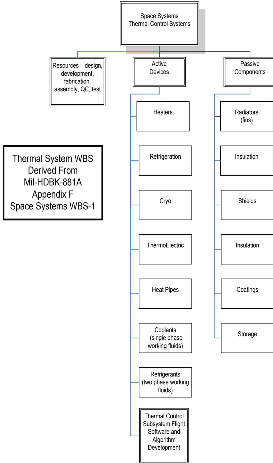
Figure 4. Thermal System WBS Derived from Mil-HDBK-881A, Appendix F, Space Systems WBS-1
