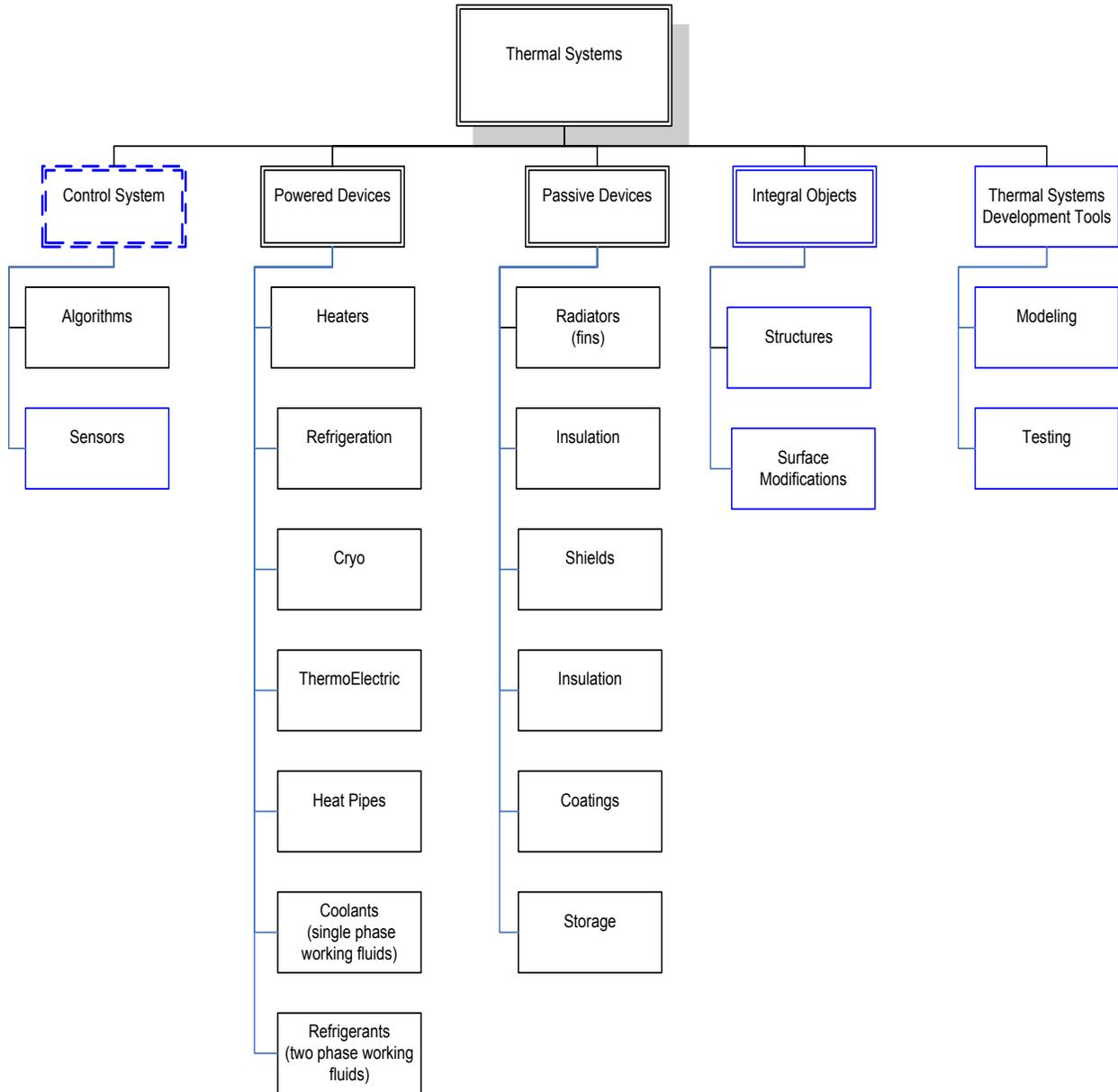
Figure 5. 1<sup>st</sup> Pass at a More Comprehensive Thermal Systems View
