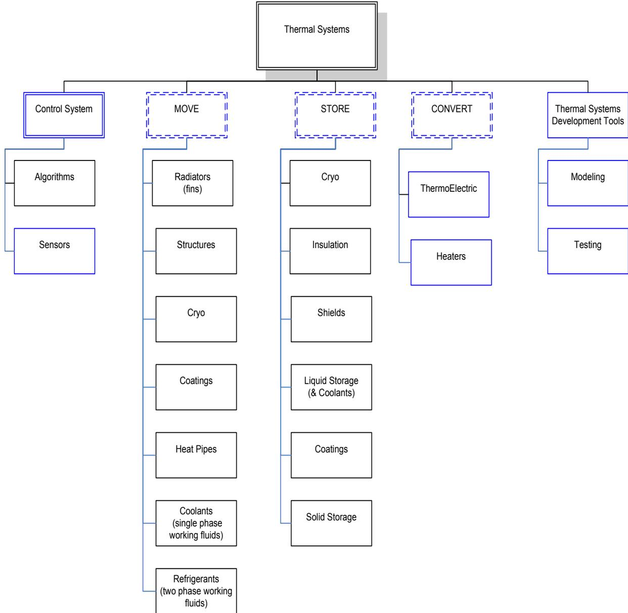
Figure 6. An Alternative “Physics Based” View of a Thermal System
