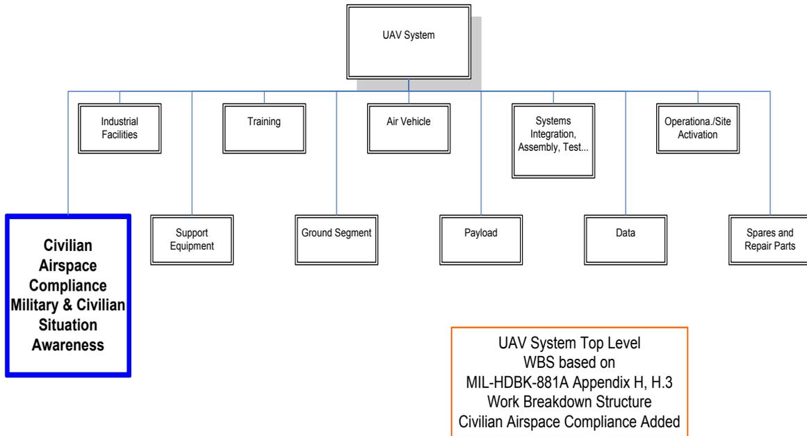
Figure 11. UAV System Top-Level WBS of Figure 10 with Civilian Airspace Compliance Added
